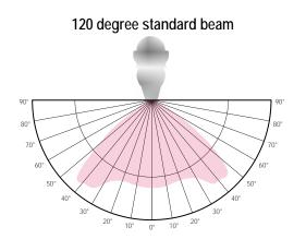
With regards to light distribution SG02 have opted for a wide beam120 degrees output. In this way you can easily obtain a perfect flat light level over bars, what makes the system also suitable for lower crop light levels.
